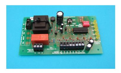
This module allows remote monitoring of up to 5 EC fans. It uses the Tacho output of the EC Fan/s. If any fan/s drop below a pre-set RPM then a fault output is generated. Fault conditions are given out by voltage free relay contacts, on board LED indication and also an analogue DC voltage.
